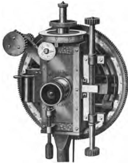
FIG. 27. — Position Micrometer By Warner & Swasey
